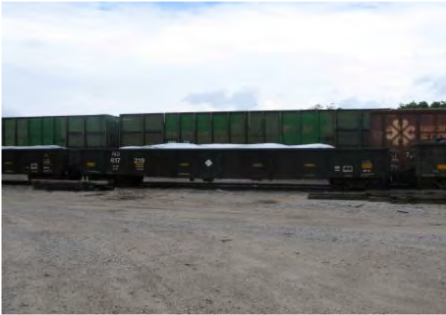
Loaded train. The gondola cars are much lower than standard bottom dump or rotary dump cars.
