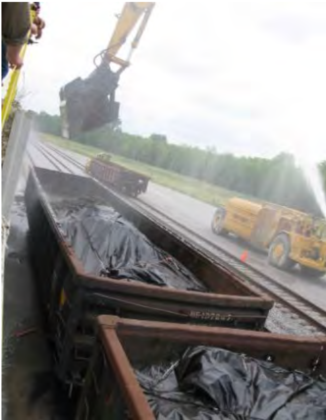
Unloading cars at Arrowhead Landfill. A water truck was used to simulate unloading during a heavy rain.
