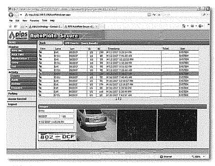
The AutoPlate Secure System enables the operator to search for a license plate and display all entry and exit information for that vehicle, or display all results against a certain database.
