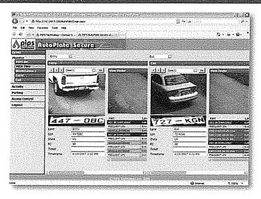
The PIPS AutoPlate® Secure ALPR Access Control System catalogs all vehicles entering or exiting an access point to a site or facility. With data provided from a PIPS ALPR camera, processor, and Optical Character Recognition (OCR) engine, the program identifies vehicles as known or unknown, or classifies them into one
