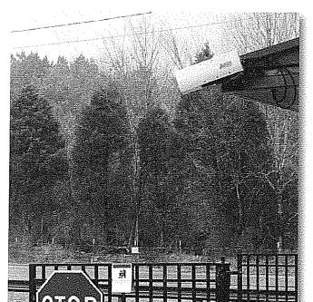
The AutoPlate Secure System provides data in real time, along with a time and date stamp, lane number, and images of both the vehicle and license plate—to either a booth attendant or to an integrated barrier or ticketing system for complete automation.
